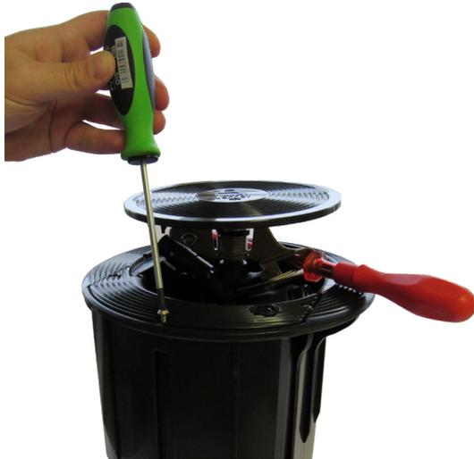
The electrical connection is thus not exposed to the soil, but is instead protectively integrated inside the sprinkler and accessible again at any time. This simplifies any search for faults and any maintenance work can be carried out at any time without any earthwork.
