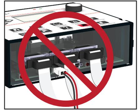
**Remember, do not connect the Molex cable and the output boards at the same time.**
